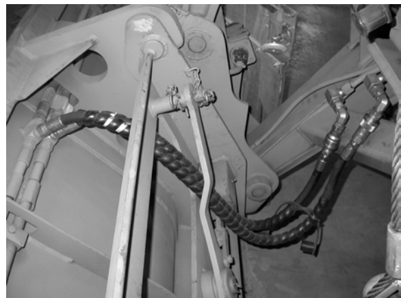
ROUTE HOSES THROUGH QUICK-HITCH FRAME AS SHOWN
